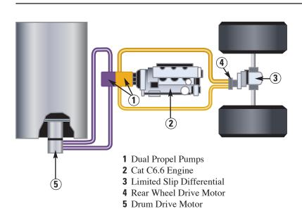
**Dual propel pumps.** Dual propel pumps provide separate, balanced hydraulic flow to the rear wheel axle and the drum drive motors. Provides superior gradeability on steep slopes and increases tractive effort in loose or poor underfoot conditions.
