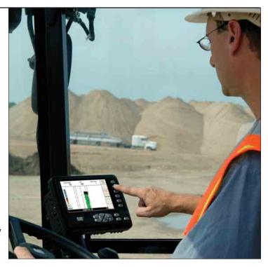
**Lower owning and operating costs.** The system will speed up the pace of the job by helping the operator determine when to move on, and lower fuel consumption by eliminating unnecessary passes.
