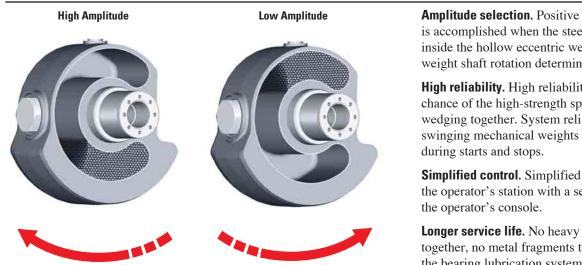
Amplitude selection. Positive amplitude selection is accomplished when the steel shot is repositioned inside the hollow eccentric weight. Direction of weight shaft rotation determines amplitude level.
