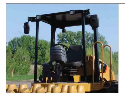
**Standard equipment.** Standard equipment includes two front-facing and two rear-facing working lights, hand rails with angled foot rests, a lockable vandalism guard and a rear view mirror.
