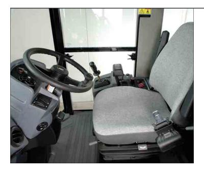
**Operational gauges.** Steering console and instrumentation gauges are infinitely adjustable within the tilt range to the desired position of the operator. Entire console tilts for simple entrance and exit.
